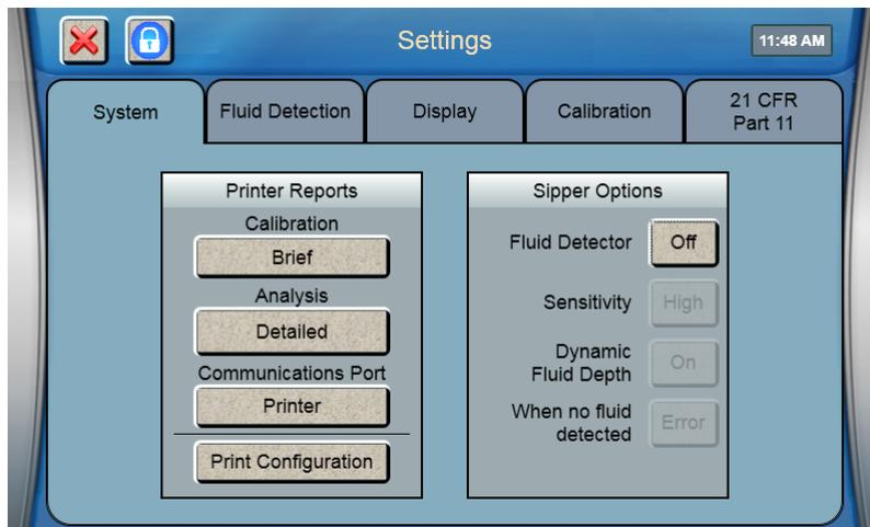
Touch the Dynamic Fluid Depth [On] button and change it to [Off] to disable sipper fluid detection and use fixed depth at sample stations.
