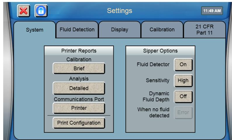
Touch the "When no fluid detected" button and select the sample fluid detection mode you prefer:
