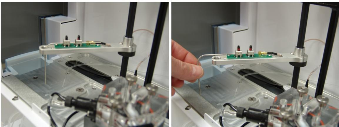
Carefully insert the long thin end of the new sipper and slide it into the mounts. Slide the sipper cone up the sipper and screw it into the sipper arm. Be sure the sipper is centered in both mounts. Tighten the mount screws gently until they contact the sipper, then tighten an additional  $\frac{1}{4}$  turn (**do not over tighten**). Connect new tubing from the Preventive Maintenance Kit to the new sipper. Install the sipper arm cover and secure using the hex screw (**do not over tighten**).
