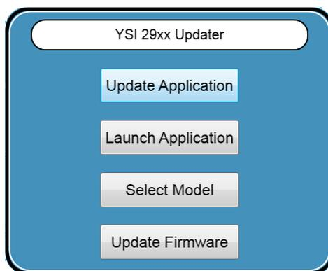
Touch the [Update Firmware] button to install the new firmware.
