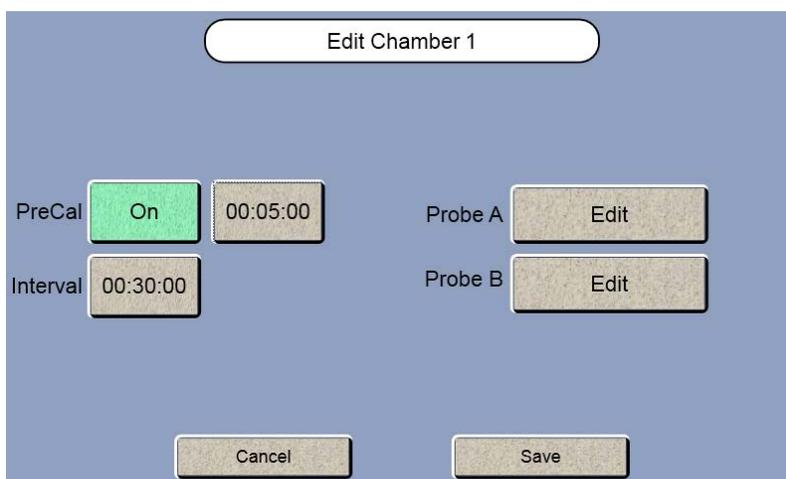
When in the monitoring mode and when the 2900 Series is stabilized in terms of calibration drift, you may elect to disable autocalibrations related to time and number of samples and use the PreCal option only.
