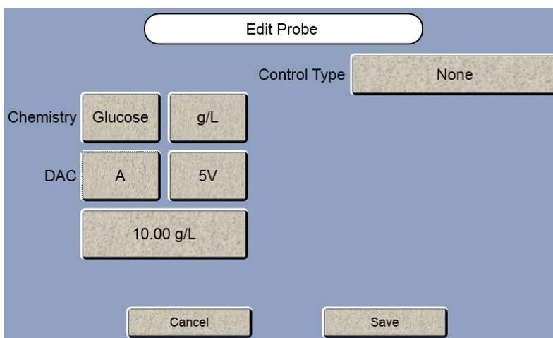
18. The Analog output can be set to 5 Volts or 10 Volts full scale. Touch the DAC [5V] button to change the Voltage to [10V].
