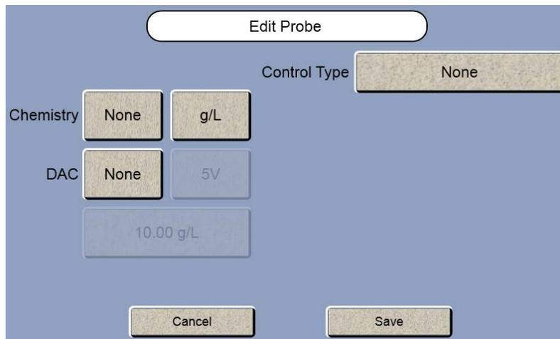
14. Touch the Chemistry [None] button and select the chemistry you are monitoring.
