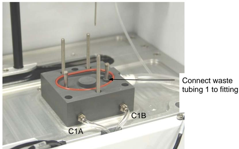
**Calibrator and Waste Tubing (Module 1)**
