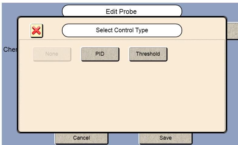
6. Select the type of control for this channel, [PID] or [Threshold], and follow the corresponding instructions in the section below.
