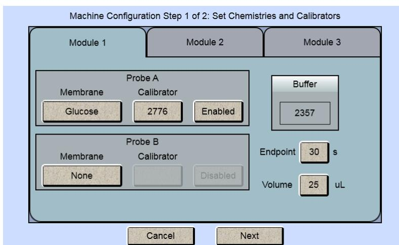
5. To run a second chemistry in module 1, touch the Probe B membrane button. Only chemistries that can be run simultaneously with your selected chemistry will be displayed.
