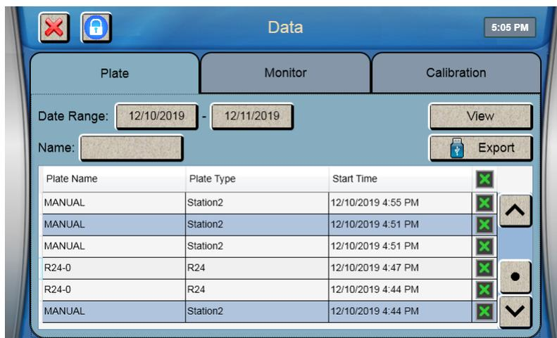
Plug a flash drive into the 2900 Series' USB port, then touch the [Export] button to send the selected sample results from memory to the flash drive.
