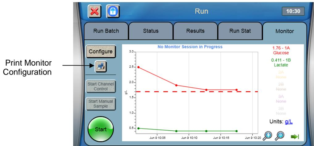
Touch the Print Monitor Configuration button to print the current monitor configuration. The configuration can then be reviewed on the YSI 2901 Printer or from the Status tab:
