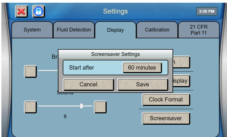
Touch the number of Minutes button next to “Start after.” Enter the number of minutes that the instrument should remain idle before enabling the screensaver, then touch [OK].
