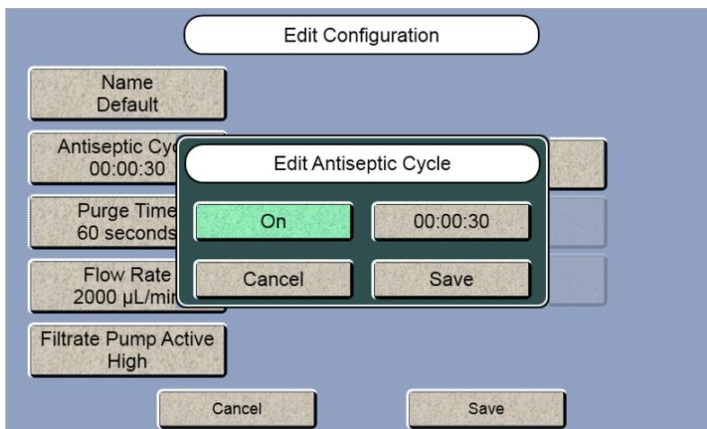
7. Touch the [On] button and change it to [Off] if you are not using an antiseptic solution.
