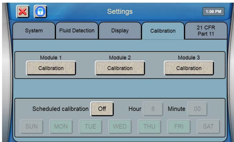
Touch the [Calibration] button for a module to display the Calibration settings for that module.
