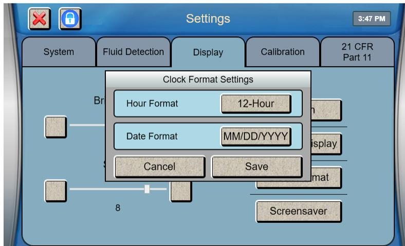
Touch the Hour Format button and select [12-hour] or [24-hour] clock format.
