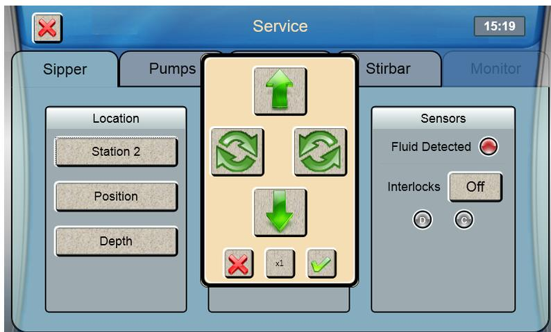
Touch  at the bottom right of the adjustment window, then touch [YES] to save the position.
