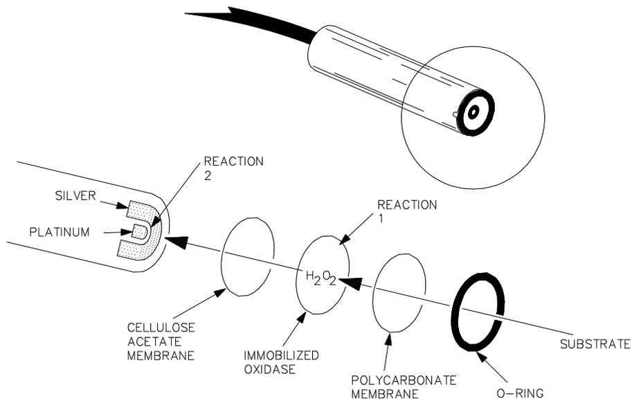
Sensor Probe and Enzyme Membrane
