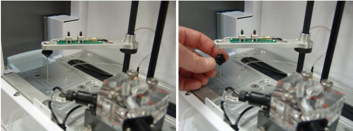
Unscrew the sipper cone, slide it down and remove it from the sipper. Loosen the two needle mount screws two turns, then remove the sipper by sliding it straight out of the mounts.
