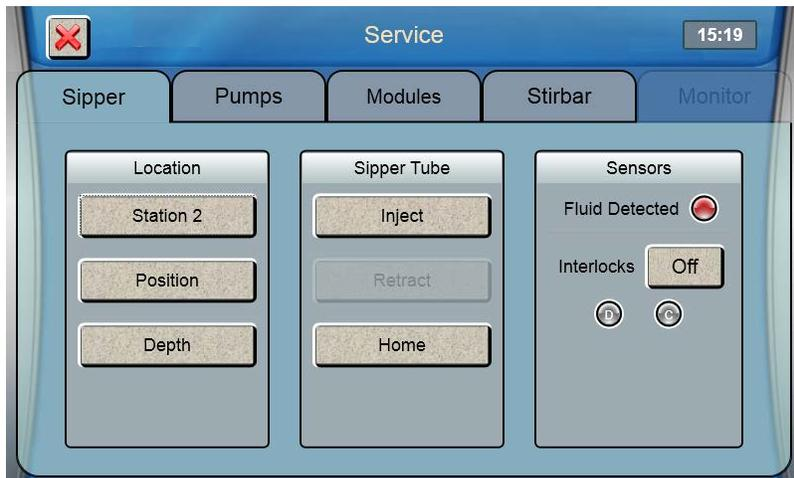
Touch the [Position] button and use the arrow buttons to align the sipper with the selected location.
