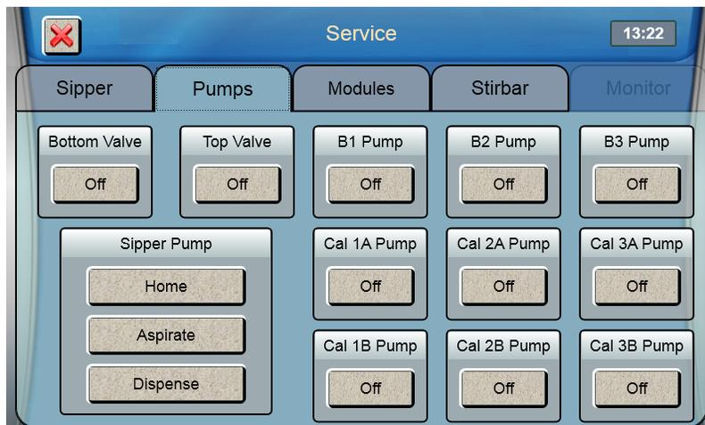
2. Touch the button under B1 Pump to turn it on.
