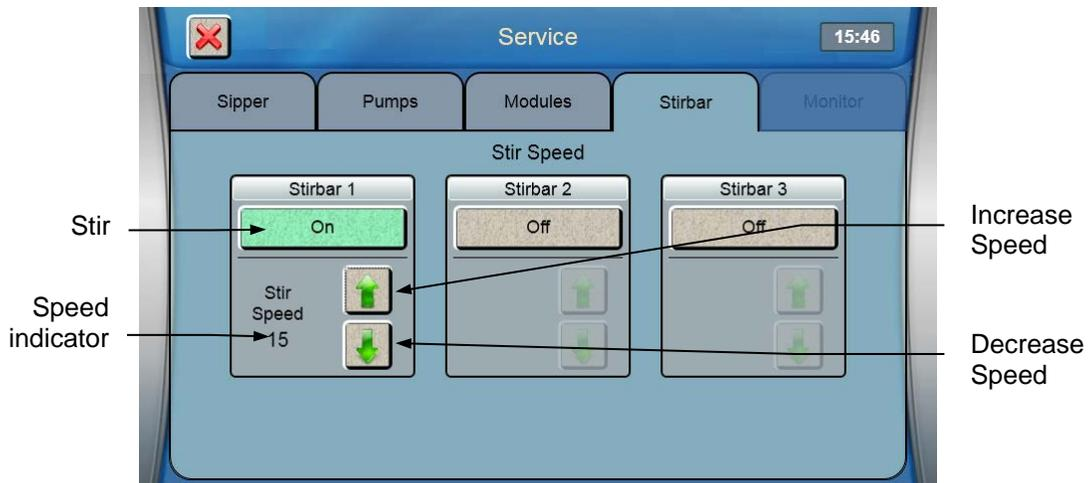
If the stir bar is jumping, use the Down Arrow Button to decrease the stir speed until the stir bar is spinning smoothly.
