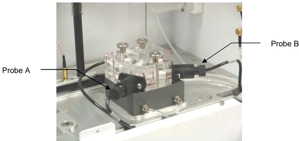
Probe A is always on the left when looking in from the side of the instrument
