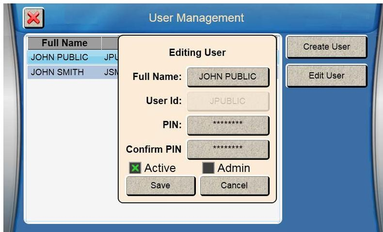
Change the Name, PIN, Active, or Admin fields as required. To disable a user, remove the X from the Active box. After you have finished making your changes, touch [Save]. Touch the [X] button to return to the 21 CFR Part 11 screen.
