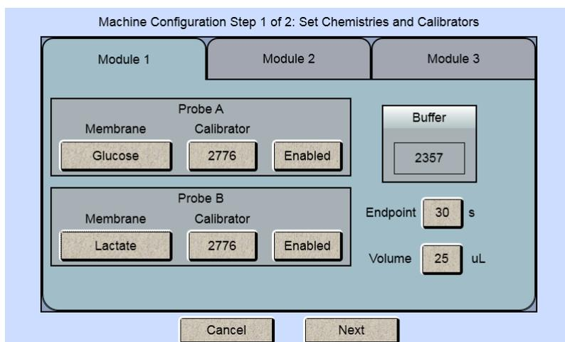
NOTE: The default Sample Volume and Endpoint for the chemistries are also displayed. **Use the default settings unless a particular application instruction specifies another value** (see Section 8 *Chemistry Setup* for details).
