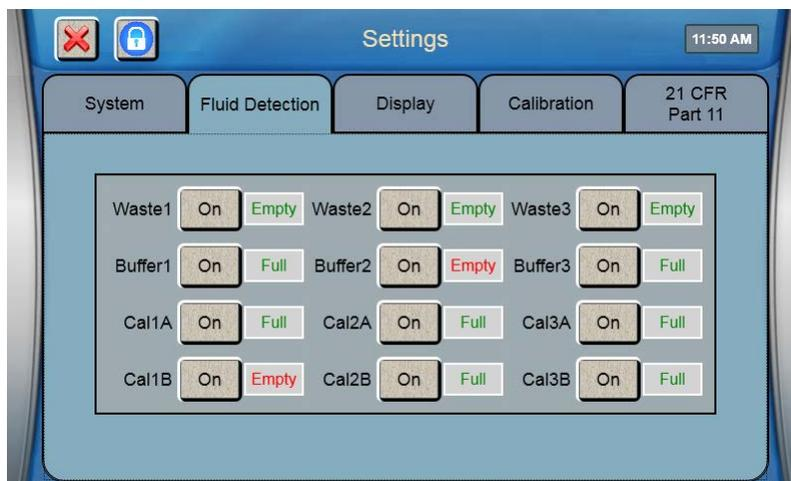
To change bottle Fluid Detection, touch the button for the bottle you wish to change. If the 2938 or 2936 Bottle Trays with Reagent Level Sensing are not installed, turn off the bottle sensors. **NOTE: When bottle sensors are off, check bottle fluid levels regularly to prevent waste fluid from backing up into sample modules.**
