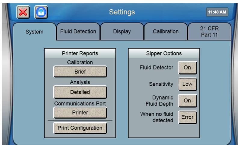
Touch the Fluid Detector [On] button and change it to [Off] to completely disable sipper fluid detection at all locations, including the calibrator wells.
