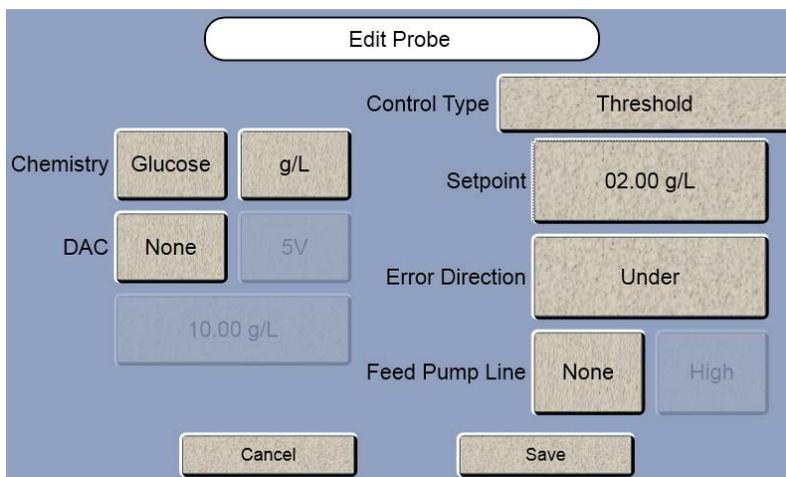
Set the Error Direction to trigger when the measured analyte value goes [Under] the threshold or [Over] the threshold.
