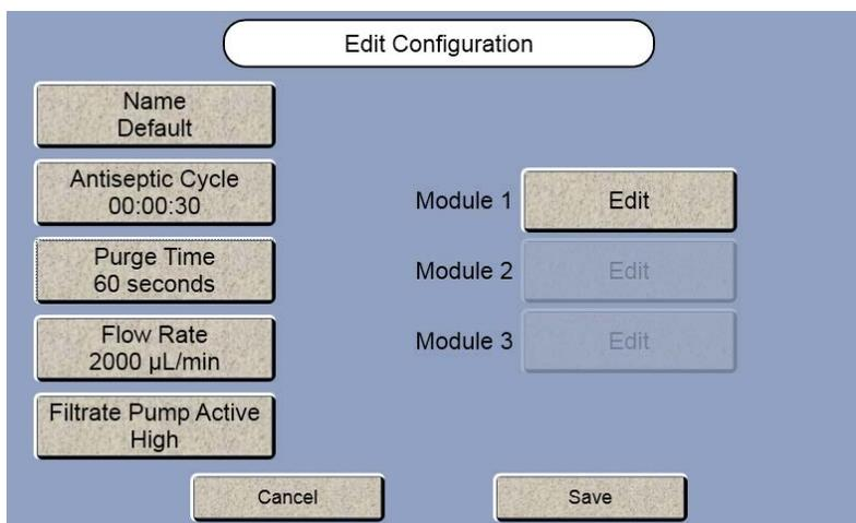
If you are using a filter on your sample line, make sure your Flow Rate does not exceed the maximum rated flow rate of your filter. If necessary, touch the [Flow Rate] button and enter the correct flow rate.
