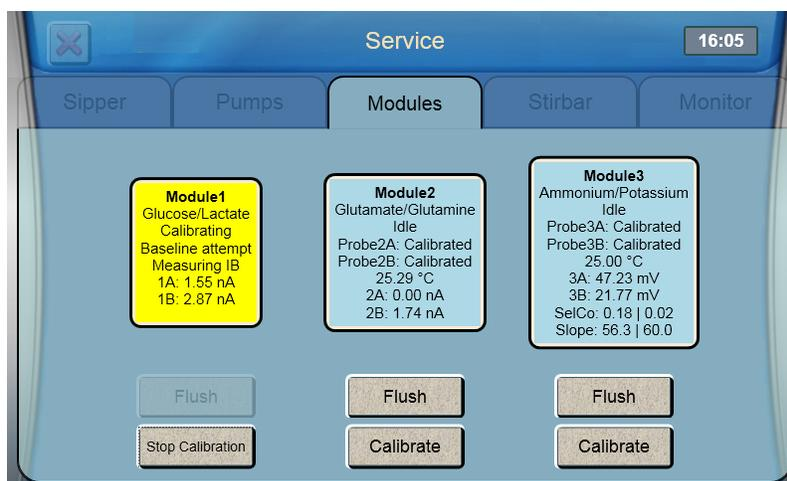
The instrument attempts to calibrate each active probe up to 5 times before aborting calibration. If calibration fails, see 11 *Troubleshooting*.
