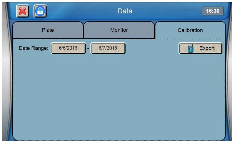
Plug a flash drive into the 2900 Series' USB port. Select a date range, then press the [Export] button to send calibration data to the flash drive.
