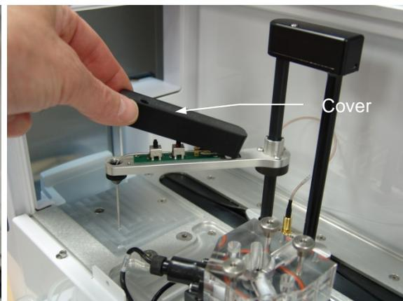
Remove the screw holding the sipper arm cover, then raise the cover up and slide it out of the sipper arm. Disconnect the tubing from the sipper.
