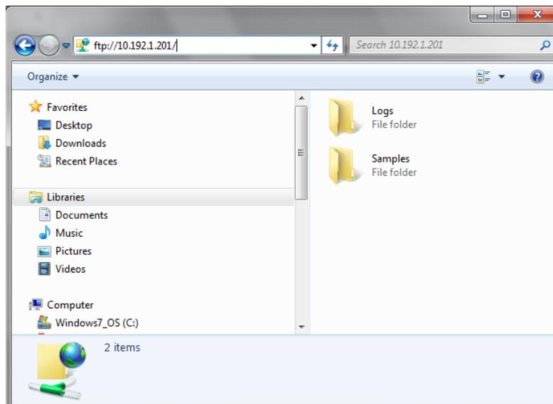
If you are unable to connect via ftp, make sure the "Passive ftp" option is **not** checked under Advanced Internet Options on your computer:
