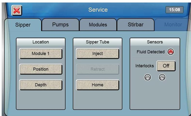
3. The Select Location screen will appear. Select [Module 1]. The sipper will move to sample module 1 and should be centered above the cone shaped opening in the top of the module. If the sipper does not move, make sure the packing material was removed.
