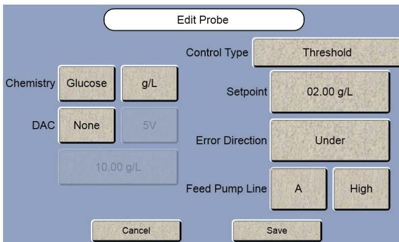
The default output is Active High (+5V). Touch the Feed Pump Line [High] button to change it to [Low] if your alarm/pump requires an Active Low signal (0V) to turn on.
