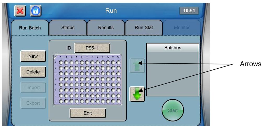
2. Touch [New] and choose from the selection of supported racks and plates. Alternatively, use the arrows to scroll through the saved racks and plates until you find the type that you are using.
