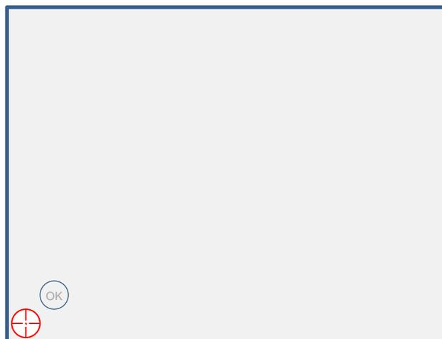
Touch the [Calibrate Display] button to enter touch screen calibration.
