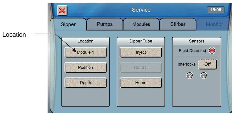
To align the sipper at other locations, touch the button under Location.
