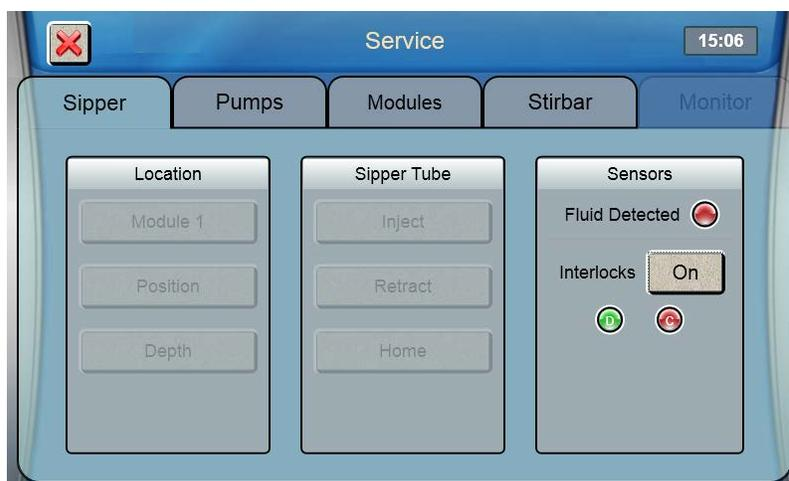
6. Touch the Interlocks [On] button and change it to [Off] to disable the safety interlock, and then press  to confirm.
