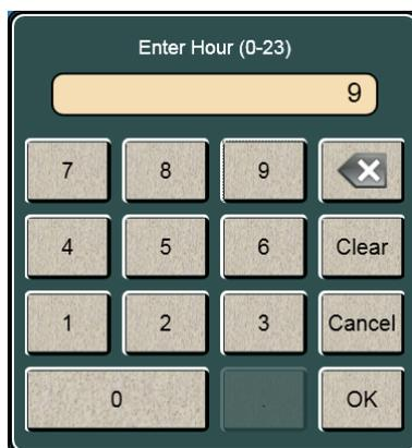
Enter the Hour each day that the instrument should calibrate in 24 hour format (0–23), then touch [OK].
