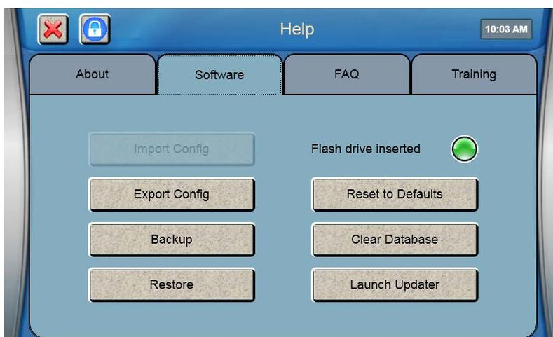
Press [Export Config] to save the current instrument configuration to the flash drive.
