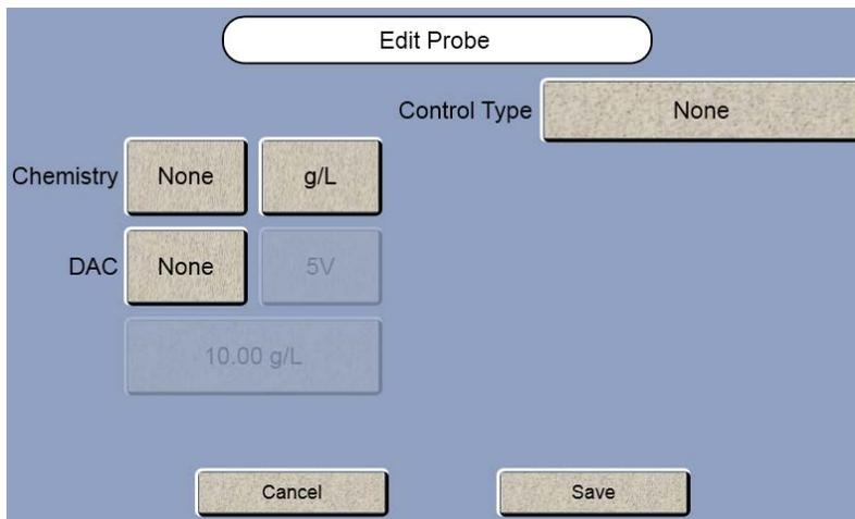
23. Enter the Chemistry and Units for Probe B. Analog output and Control can also be set for Probe B.
