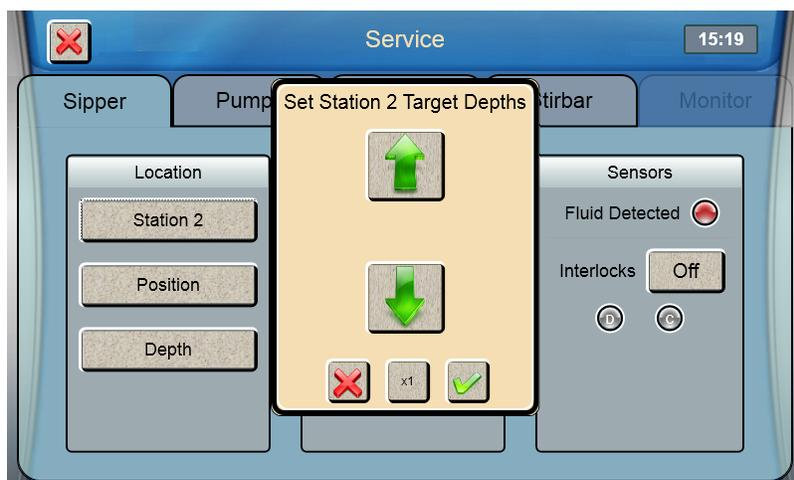
Touch  at the bottom right of the adjustment window, then touch  to confirm saving the position.
