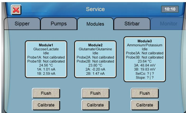
The Modules tab displays the status of the probes, probe current for each enzyme probe, voltage for each ISE, and the temperature. The probe current is expressed in nA (nanoamperes,  $10^{-9}$  amperes), a very low level of electrical current.
