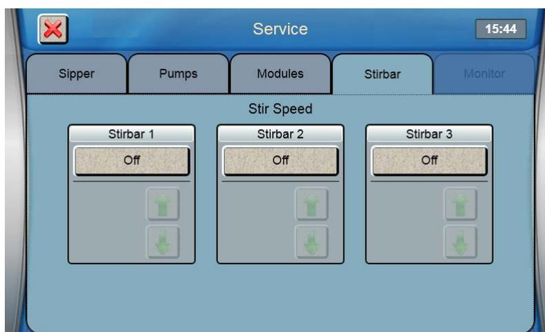
The StirBar screen is used to adjust the speed of the stir bar.
